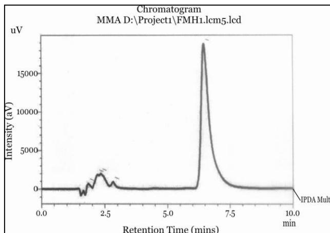
**Fig. 2:** Typical chromatogram of standard monomer concentration (1600ppm).
