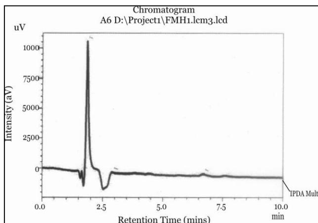
**Fig. 3:** A sample chromatogram of specimen after soaking in distilled water for 6 hours' time interval.
